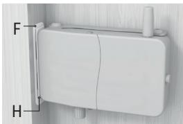
**2.** Next to the adhesive spacer (H), position the trim (F) on the door frame. The spacer marks the minimum distance between the lock and the trim. If both these parts are not at the same height, you must use the shims (C) to wedge the lock as shown in step 4.
