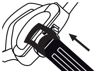
4. Rotate following the groove until you reach the locking position. Once you have done this, you must be blocked to fix the tube.
