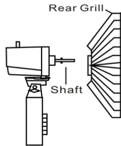
Slide blade on motor Shaft
