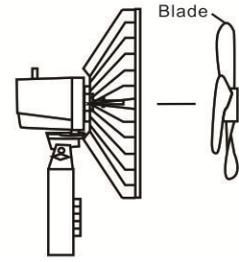
Screw blade cap on shaft by turning counter clockwise
